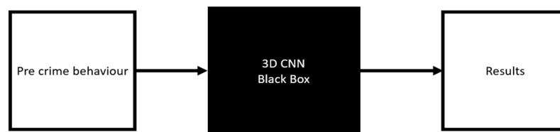
Figure 1. The black box model for shoplifting detection, where a raw video sequence is used to train a black box algorithm (such as a 3D CNN as in [6]) to detect suspicious individuals. The nature of these models makes them difficult to interpret and susceptible to bias in the training data.
