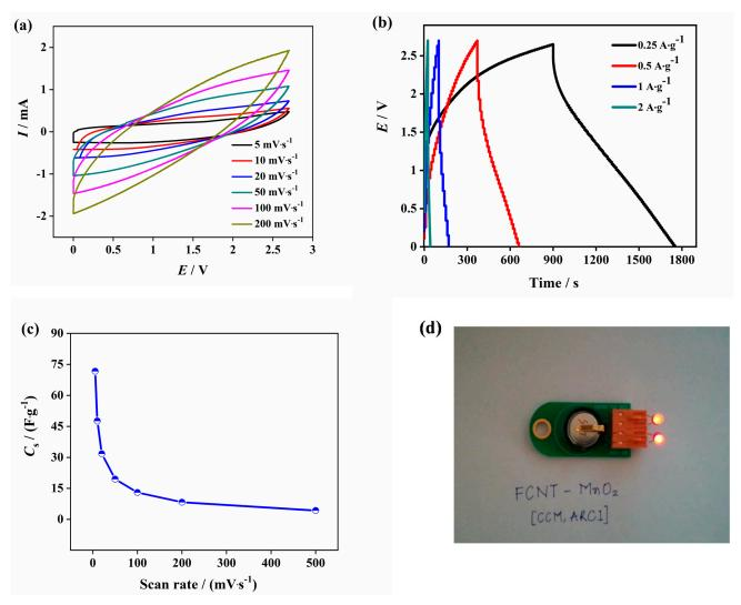
**Figure 5.** Electrochemical analysis of FCNT-MnO<sub>2</sub> in the organic electrolyte (1 M TEABF<sub>4</sub> in Acetonitrile (1:1)) (a) CV, (b) GCD, (c) specific capacitance from CV, and (d) LED glowing from FCNT-MnO<sub>2</sub> cell.
