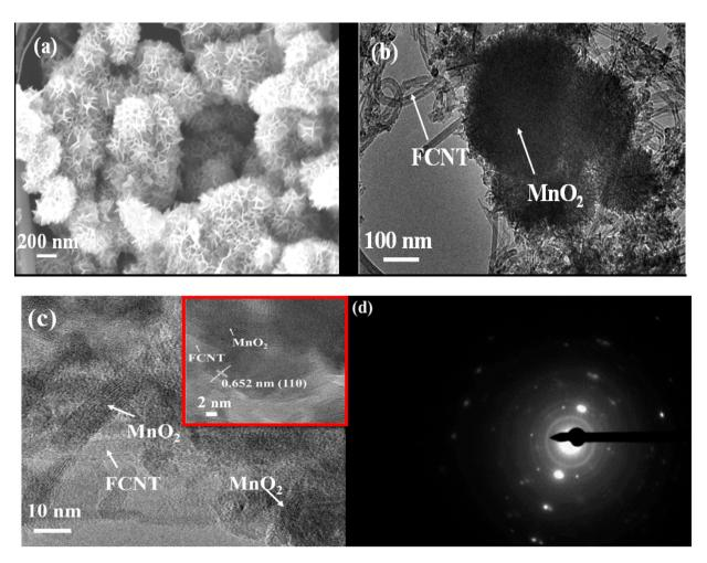
**Figure 2.** (a) FESEM of FCNT-MnO<sub>2</sub>, (b) TEM analysis of FCNT-MnO<sub>2</sub>, (c) HRTEM of FCNT-MnO<sub>2</sub> with inset showing the lattice spacing of MnO<sub>2</sub> in the hybrid FCNT-MnO<sub>2</sub>, and (d) SEAD pattern of FCNT-MnO<sub>2</sub>.
