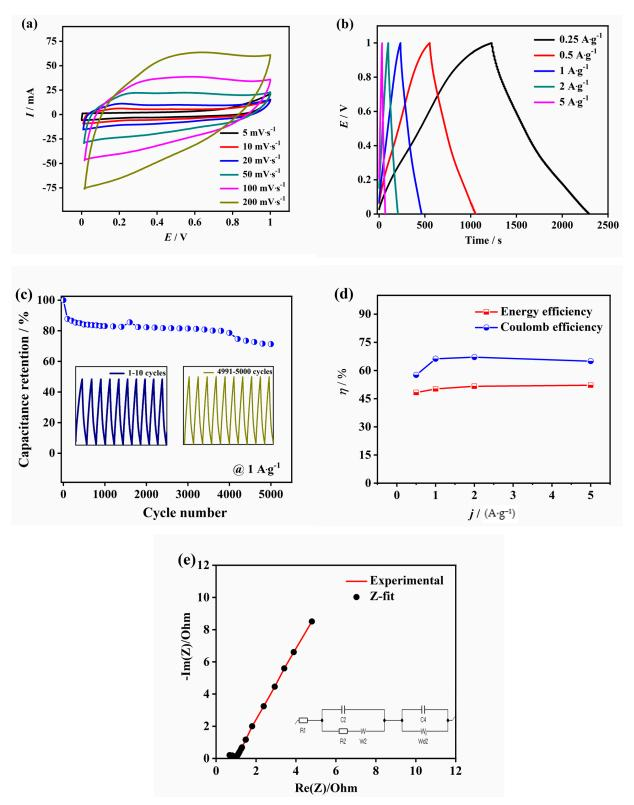
Figure 4. Electrochemical analysis of FCNT-MnO<sub>2</sub> in a two-cell configuration with 3 M KOH electrolyte ( $\mathbf{a}$ ) cyclic voltammetry, ( $\mathbf{b}$ ) galvanostatic charge-discharge, ( $\mathbf{c}$ ) cyclic performance from GCD, with inset showing first and last 10 cycles of 5000 cycles, ( $\mathbf{d}$ ) coulombic efficiency and energy efficiency vs. current density plot, and ( $\mathbf{e}$ ) Nyquist plot of experimental data and Z-fit, with its corresponding equivalent circuit.
