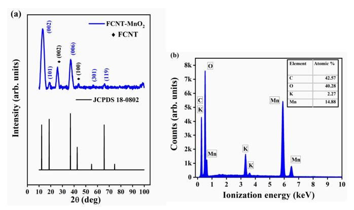
Figure 1. (a) XRD pattern of FCNT-MnO<sub>2</sub> and (b) energy dispersive x-ray (EDS) spectrum of FCNT-MnO<sub>2</sub>.
