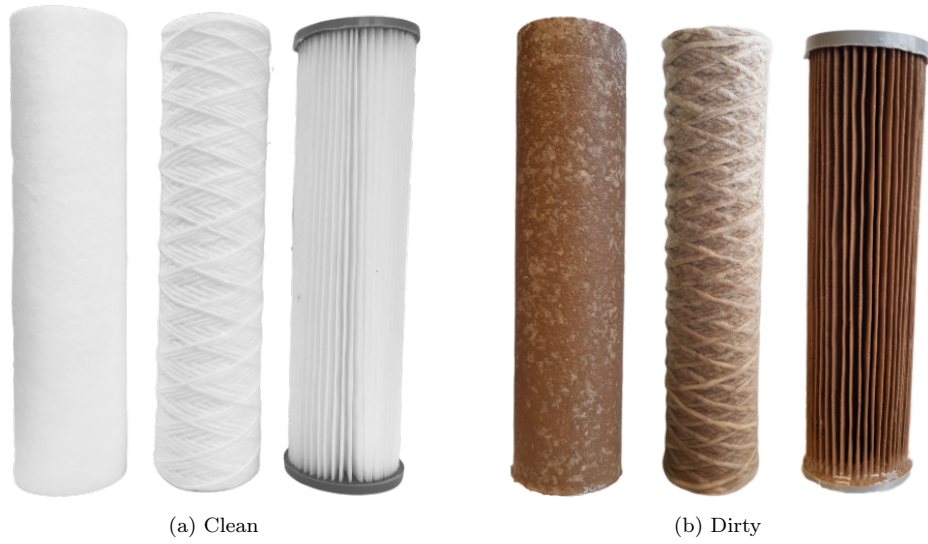
Figure 6: The three types of cartridge filter elements used in this study: spun (left), wound (middle) and pleated (right).
