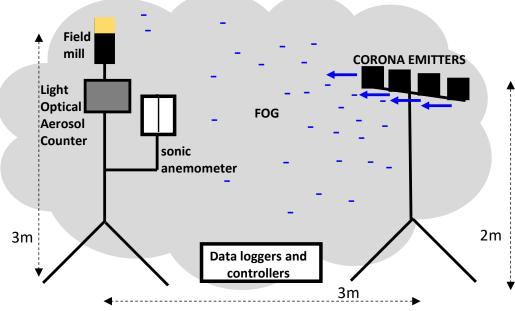
Fig 1. Practical (a) and functional (b) arrangement of apparatus at Sonning Farm, in light fog. The left-hand "measurements" mast carries a sonic anemometer, electric field mill, and the Light Optical Aerosol Counter (LOAC). The right-hand "emitter" mast carries a horizontal array of corona emitters. (A four channel Optical Cloud Sensor, OCS was also mounted at the top of the emitter mast, directed across the ion emission region.)
