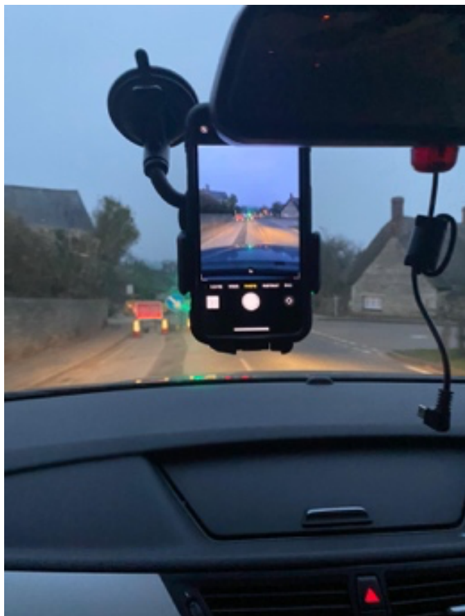
Figure 24: Smartphone placement at the windshield
