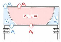
Figure 3. Schematic of two-zone combustion model
