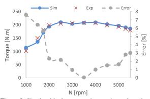
Figure 9. Simulated brake torque via experimental results for EF7TC
