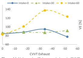
Figure 14. Volumetric efficiency variation via CVVT
