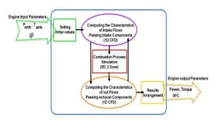
Figure 2. Schematic of one-dimensional component model with a zero-dimensional combustion sub-model
