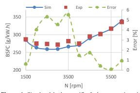
Figure 6. Simulated brake specific fuel consumption via experimental results for EF7NA
