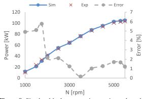
Figure 8. Simulated brake power via experimental results for EF7TC
