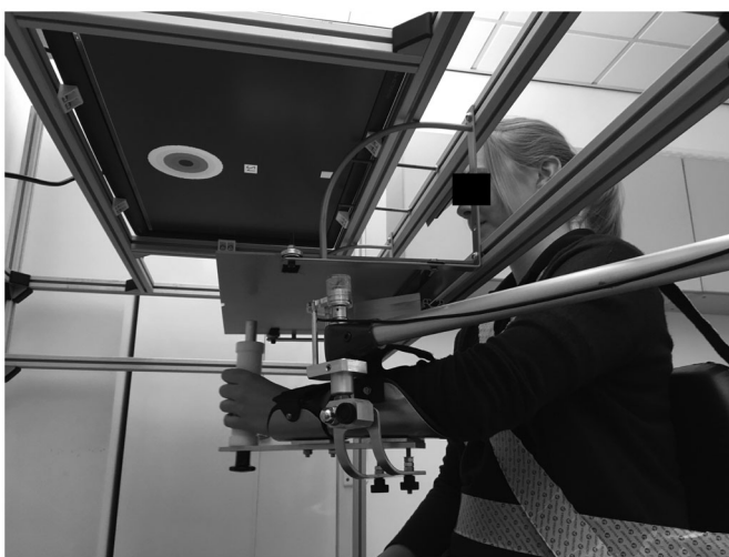
Figure 1. Training set-up. Participants were seated with forehead, trunk and shoulder support. The weight of the arm was fully supported and the hand was strapped to the handle if required. Participants were unable to see their hand but were provided with feedback of the hand location and the reaching target by an image projected on a screen.
