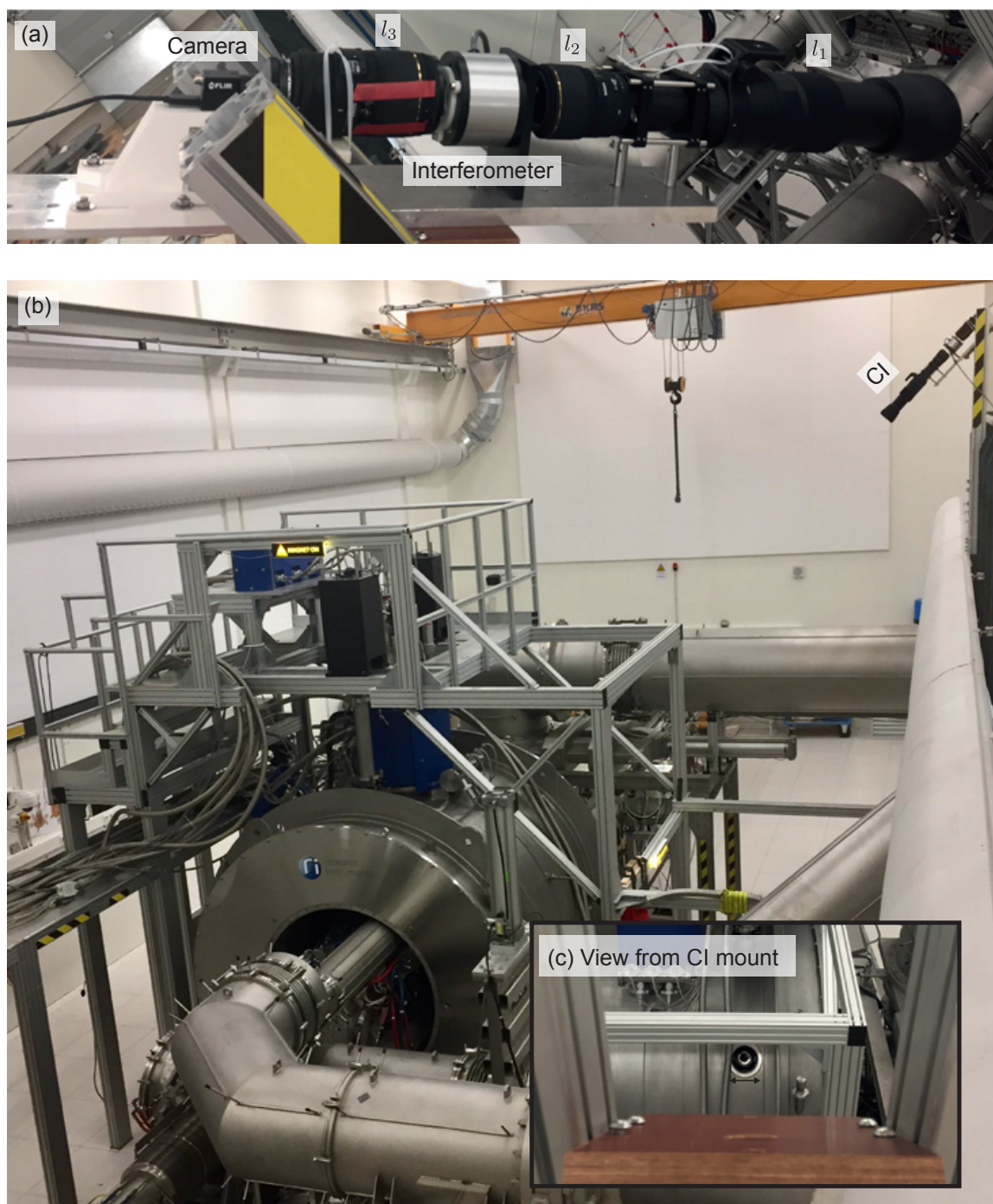
Figure 5.16: (a) The Magnum-PSI machine hall. The coherence imaging instrument is mounted to the railing of a mezzanine area, and can be seen in the upper right corner. (b) The CI instrument. (c) View from CI mount
