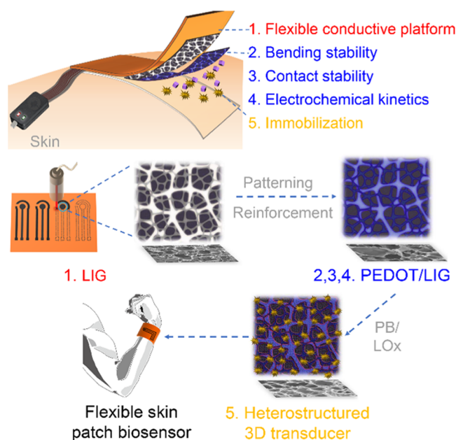
Scheme 1. Schematic Diagram of the Flexible Skin Patch Biosensor
