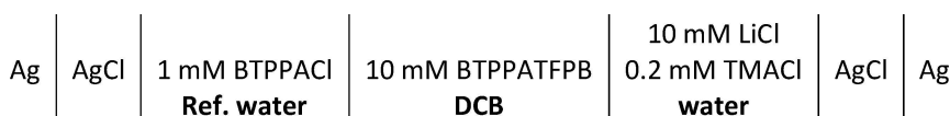
Scheme 2. The composition of the ITIES cell used to study the transfer of TMA + ion. 0.2 mM NaPF 6 in aqueous phase was used to study the transfer of PF 6 - ion.
