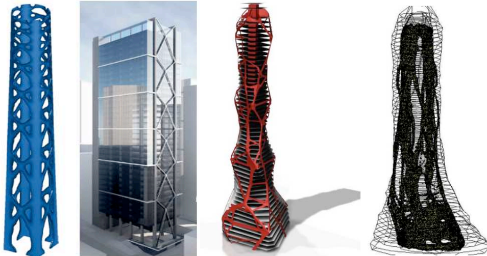
Fig. 2. Structural topology optimisation techniques on buildings (Stromberg et al., 2010; Beghini et al., 2014; Kingman et al., 2015).
