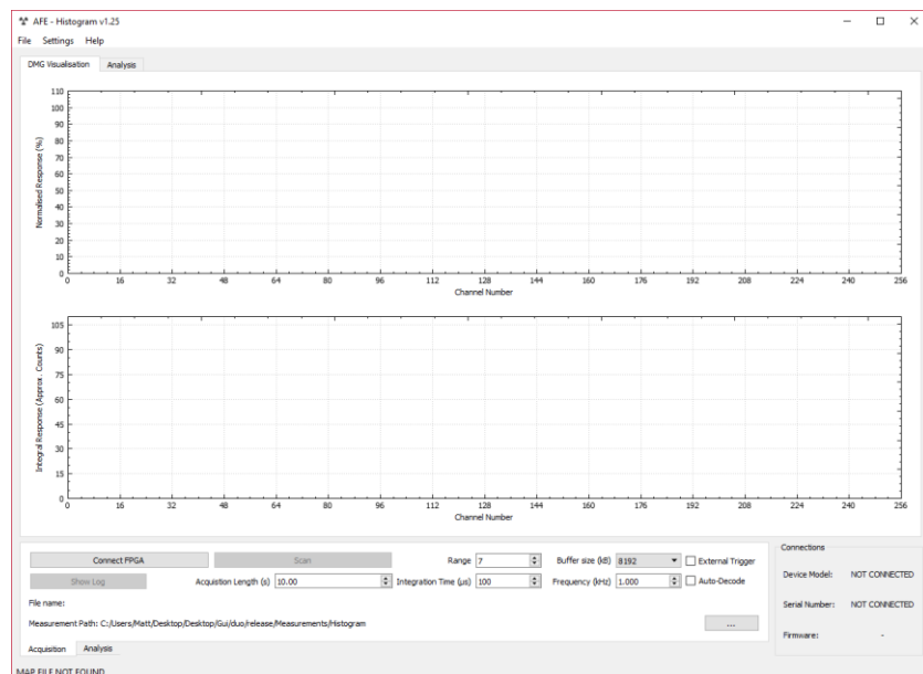
Figure 2.17 The AFE-Histogram graphical user interface (GUI) for acquisition, visualisation and analysis of sDMG measurements.
