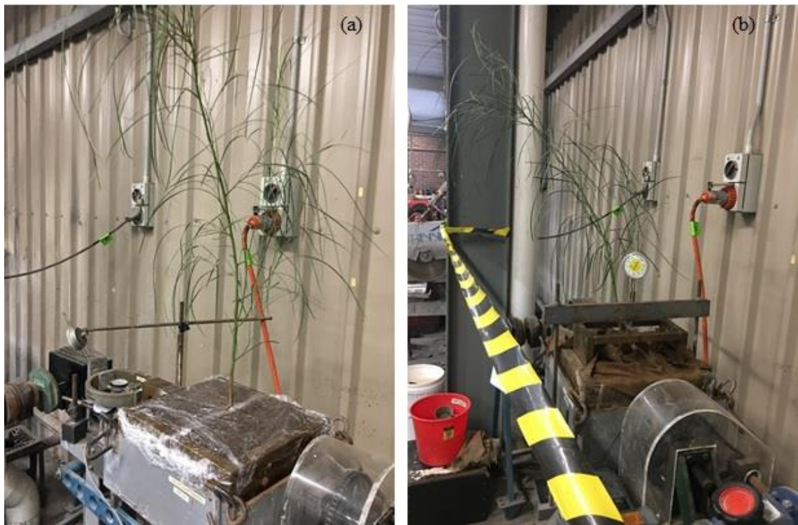
Figure 3.11 Moisture evaporation control using cling wrap and wet gunny sacks
