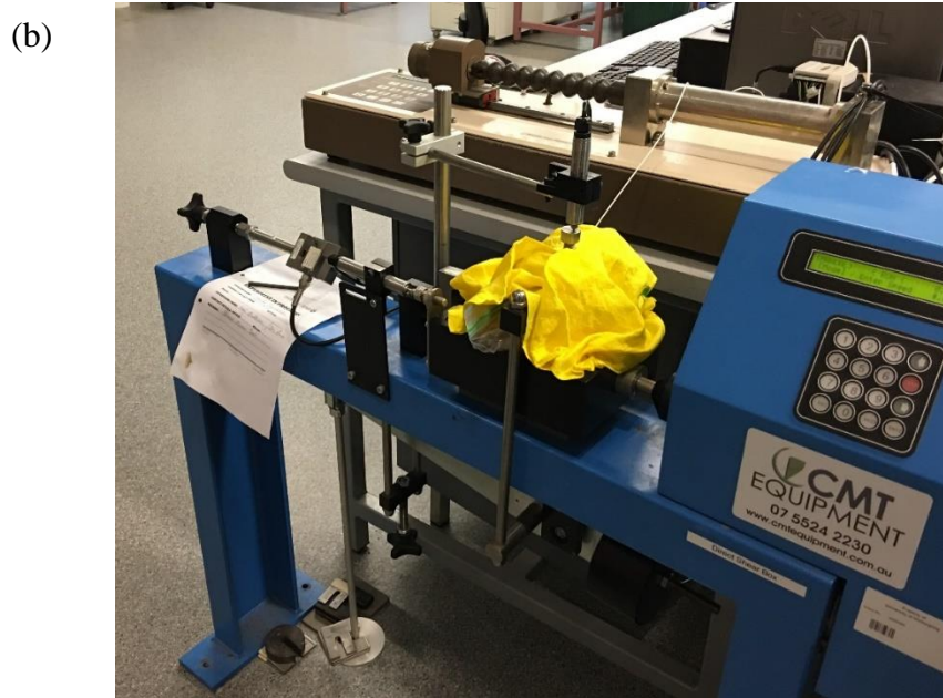
Figure 3.5 Direct shear box (60 x 60 x 40 mm), (a) schematic diagram with instrumentation and (b) an image of the direct shear box
