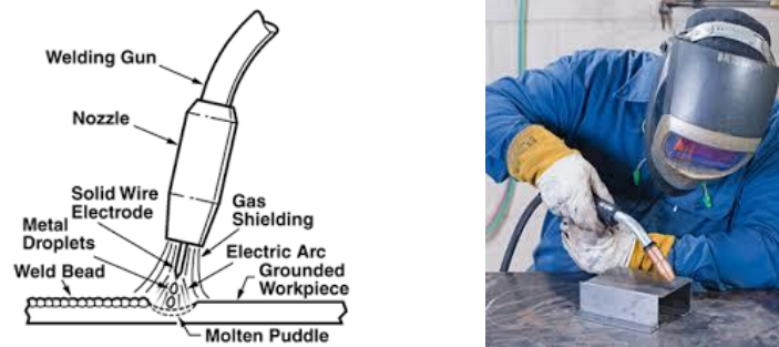
Figure 1.12 GMAW torch for manual welding [43][151]
