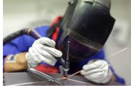
Figure 1.11 Water cooled GTAW torch for manual welding [43][150]
