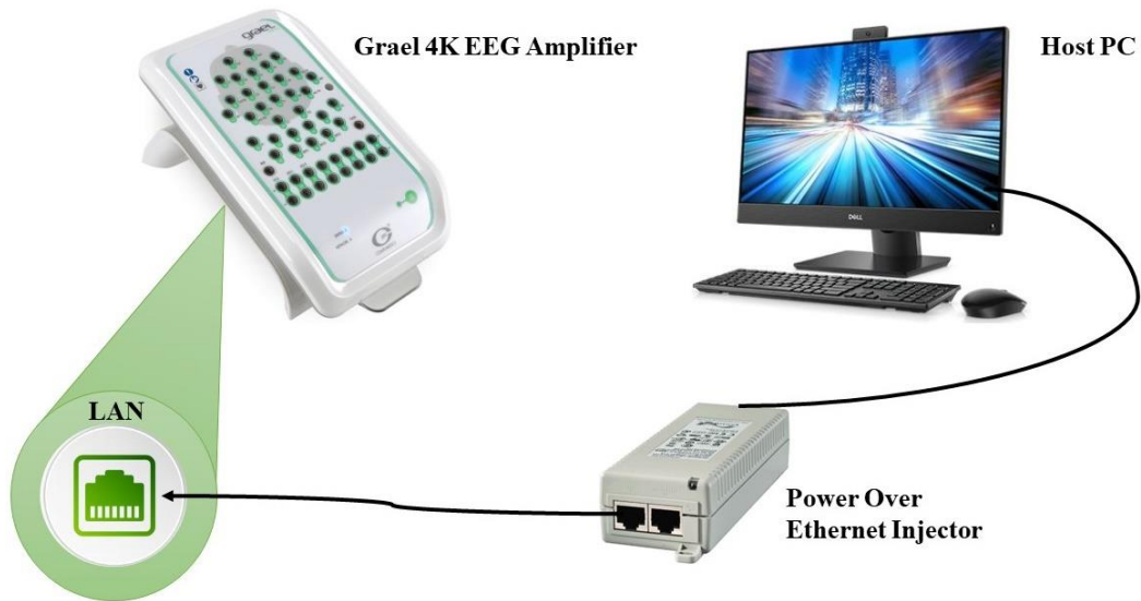
Figure 3.2: Connection of GraeL 4K EEG amplifier to host PC
