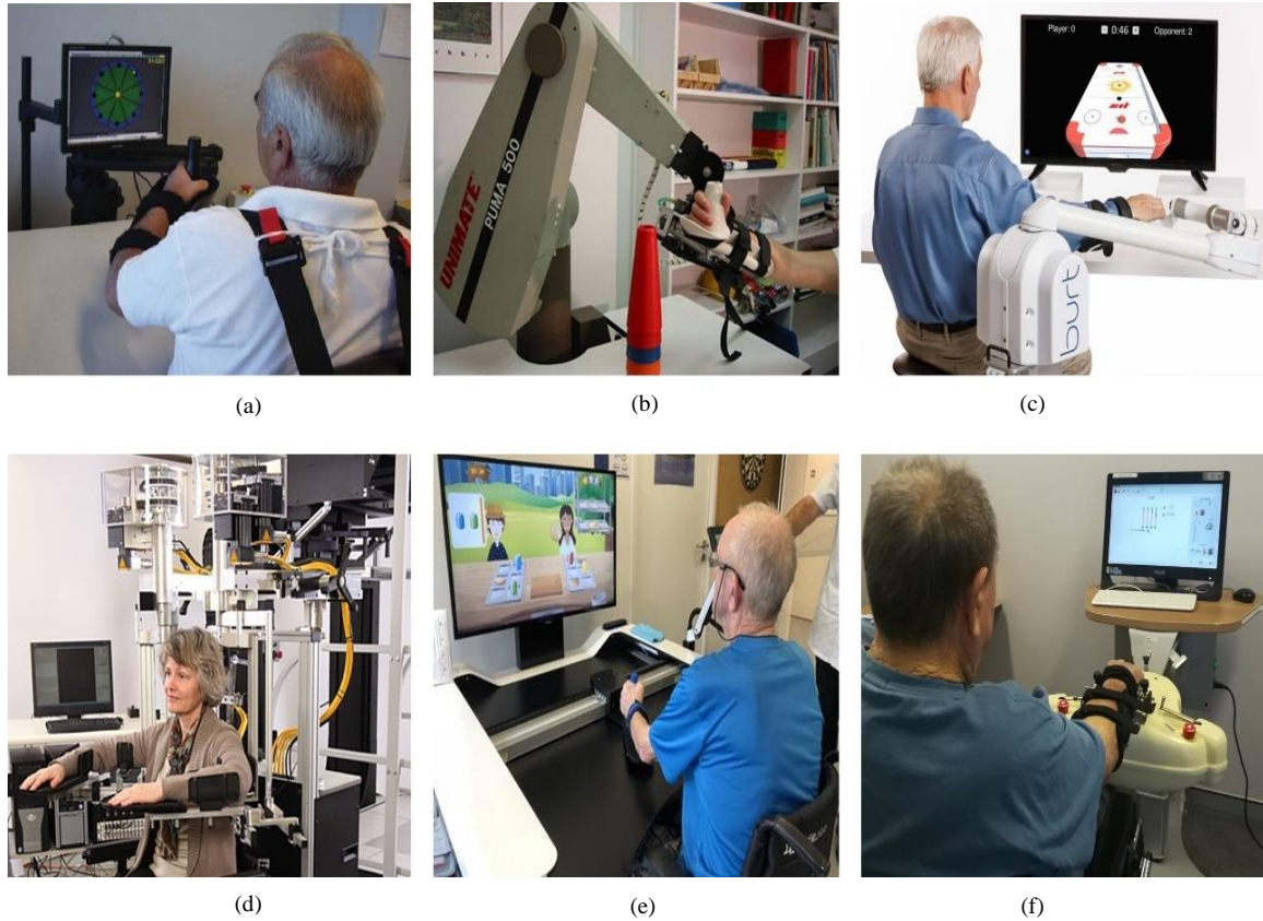
Figure 1.3: End-effector devices; (a) InMotion [49], (b) MIME [50], (c) Burt [51], (d) Kinarm [52], (e) REAplan [53], (f) AMADEO
