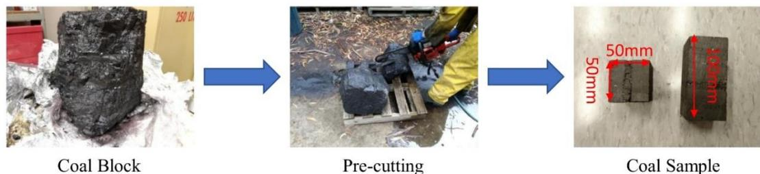
**Figure 9. 1 Coal specimen preparation**
