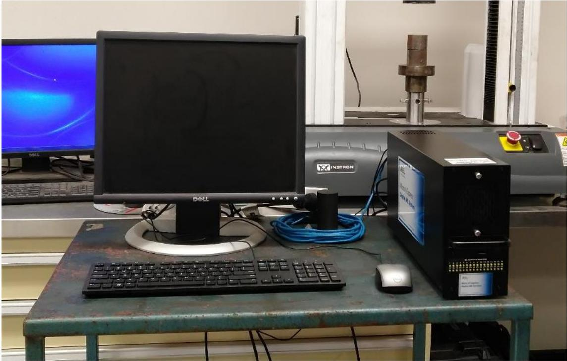
**Figure 8. 3 AE monitoring system**
