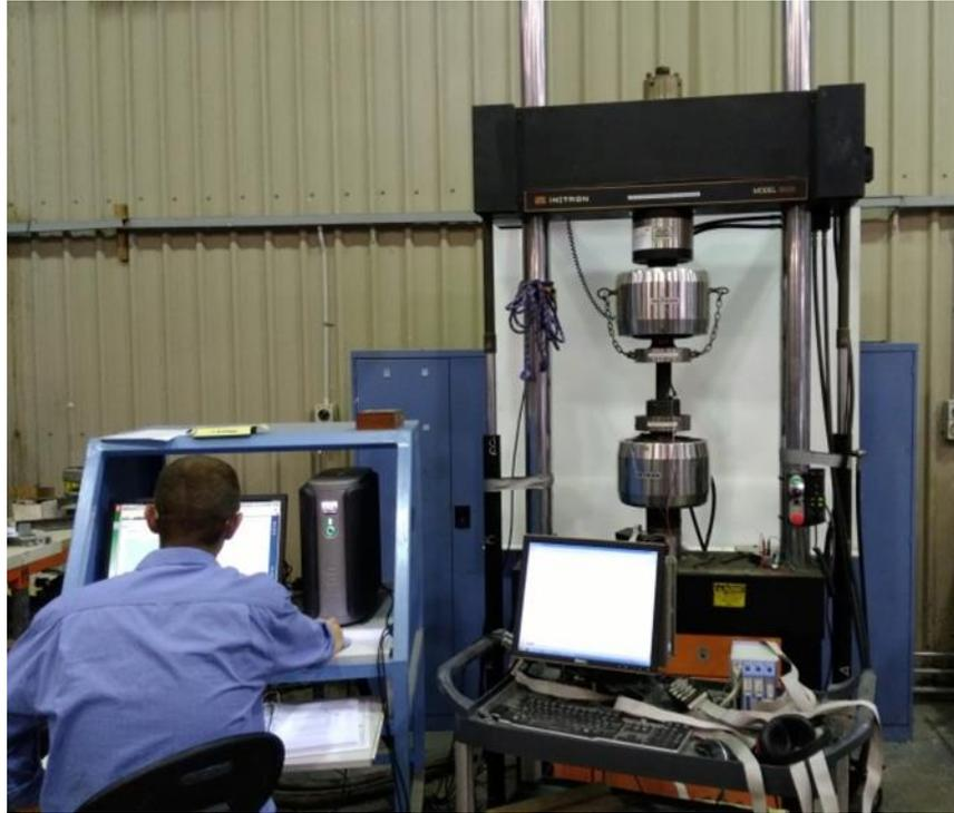
**Figure 4. 3 Universal rock testing system**
