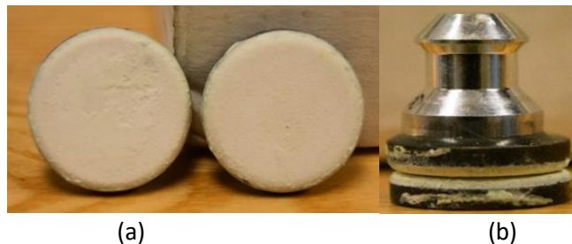
Fig. 11 (a) YSZ coated button cell samples, (b) Adhesion tester prep with the button cells and sand slurry post-sintered in the furnace
