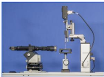
Fig. 7(a) Dynamic Contact angle measurement device
