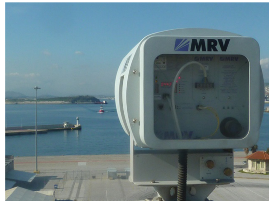
Fig. 2. The MRV TS5000/155 FSO system on the roof of HNA’s building. On its left is shown the Psittalia island where is located the second FSO system.
