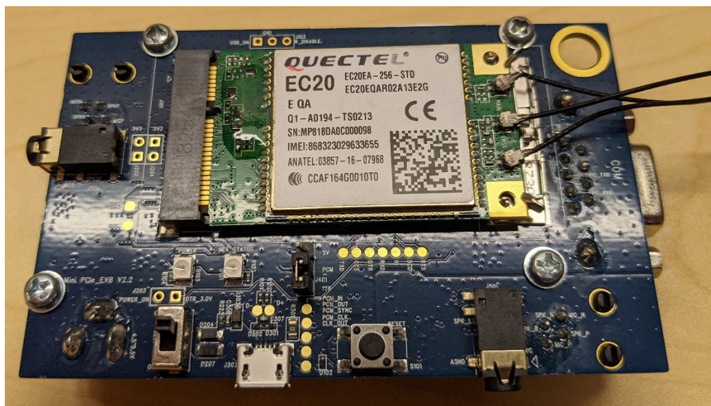
Figure 14. Quetel EC20 Modem in Developer Board
