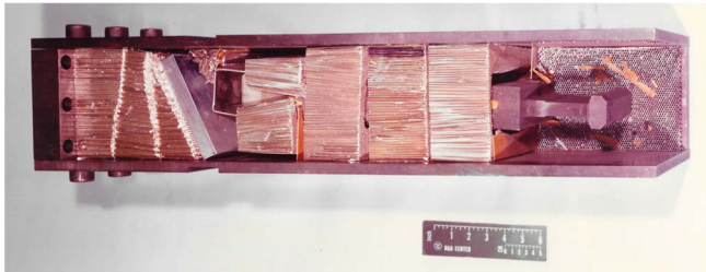
Fig. 11. Top view of the switch projectile stopped in the catch box.
