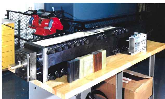
Fig. 9. 1.5 MA switch assembly.
