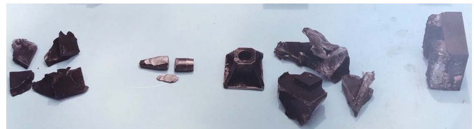
Fig. 23. Recovered launch package fragments from Test 3.
