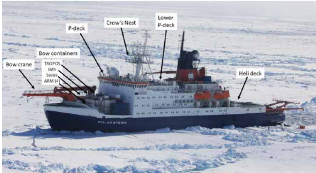
Figure 1. Polarstern embedded in sea ice, with key installation locations annotated.
