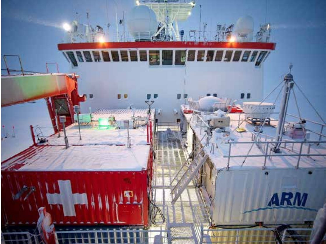
Figure 5. Polarstern bow with ARM laboratory containers and equipment visible, including installations above the bridge. Early March 2020. Photo: Michael Gutsche.
