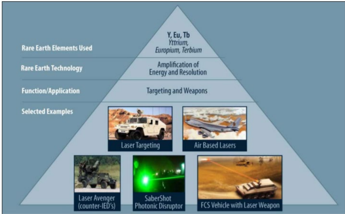
Figure 5. Rare Earth Elements in Targeting and Weapon Systems. Adapted from Grasso (2013).
