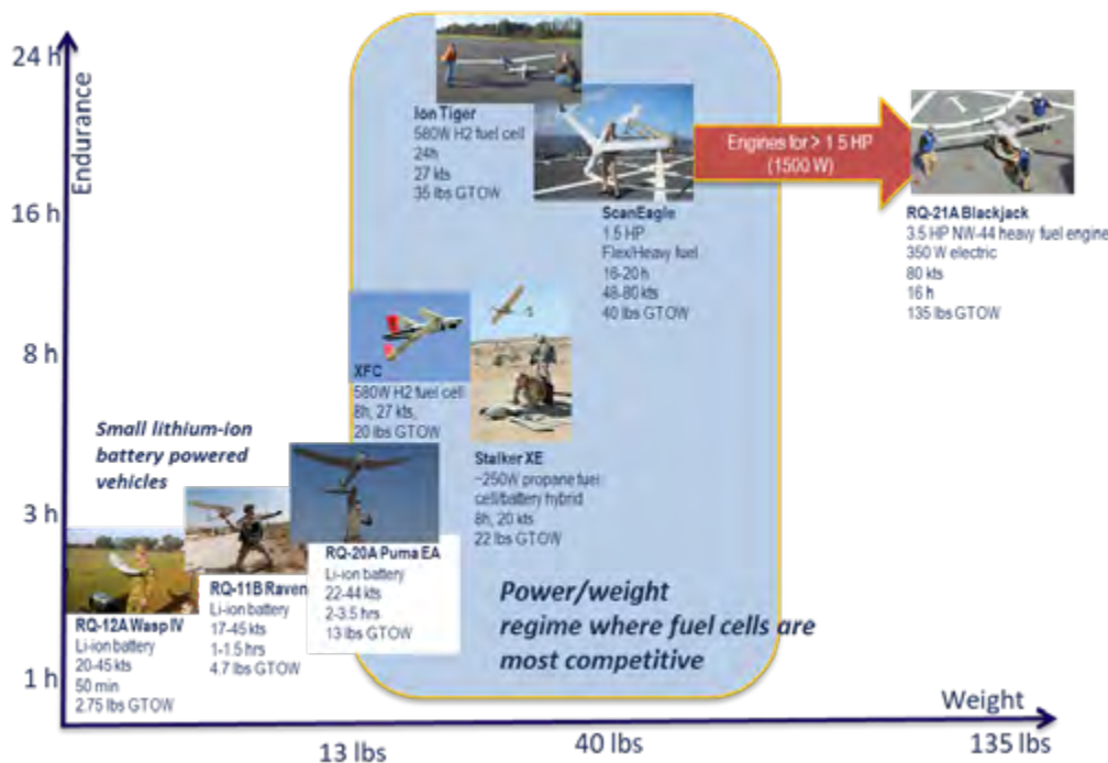
Figure 3. Tier 1 to tier 3 battery, fuel cell, and engine-powered UAS: comparison of propulsion/energy source, speed, endurance and gross takeoff weight (GTOW).
