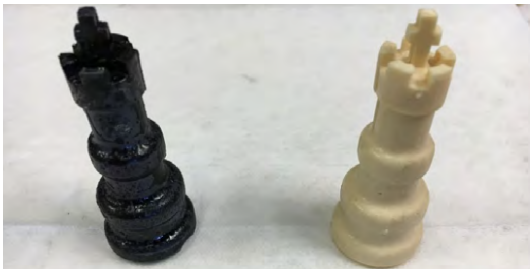
Figure 11. Chess pieces cast with explosives.
