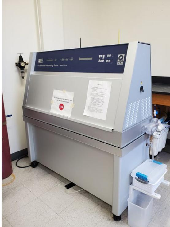
Figure 16. Q-Lab QUV/se Accelerated Weathering Tester
