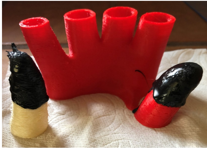
Figure 17. PVA and PLA parts with neoprene gel coating
