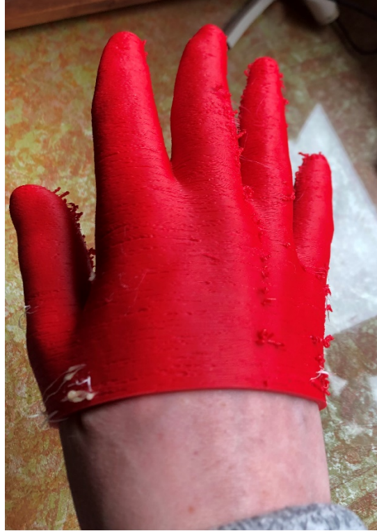
Figure 15. TPU glove with attempted PVA wall on hand
