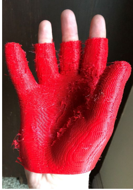
Figure 13. Partial glove with TPU after PVA dissolved away
