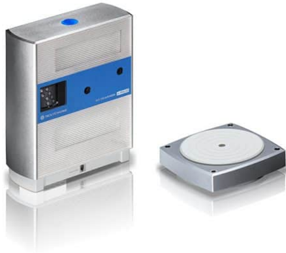
Figure 5. NextEngine 3D Laser Scanner used. Source [18].
