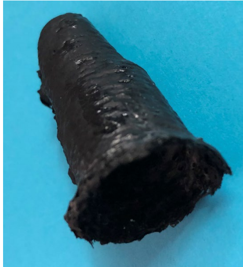
Figure 18. Neoprene gel coating after dissolving PVA
