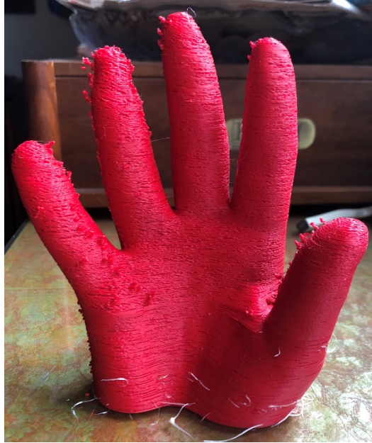
Figure 14. TPU glove with attempted PVA wall
