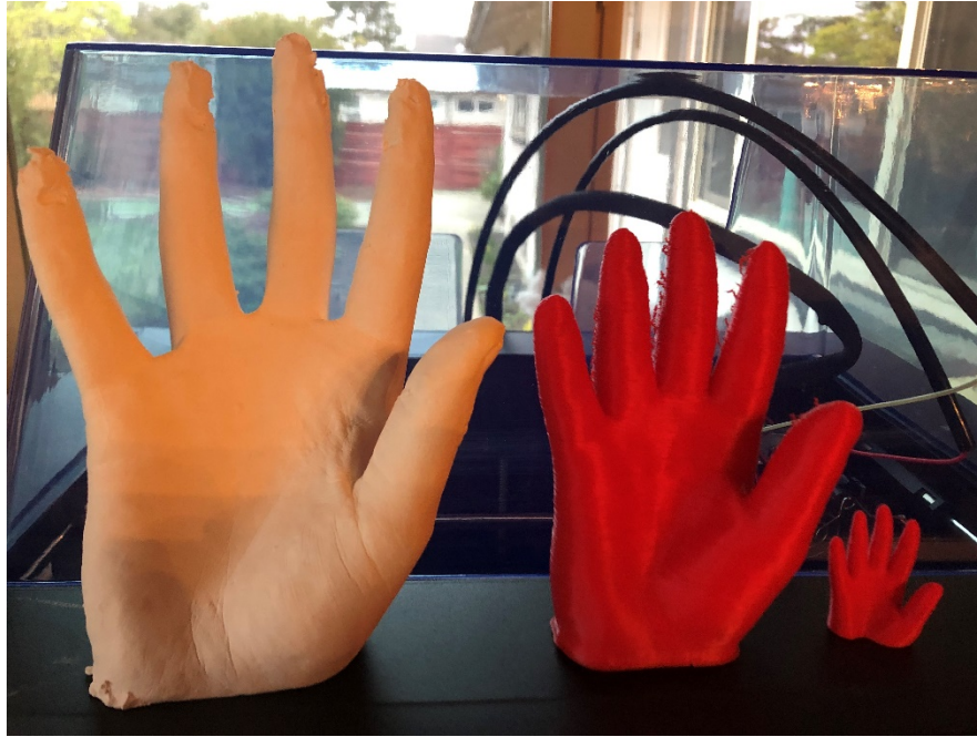
Figure 10. Cast hand, 70% scale PVA print, and 25% scale TPU print
