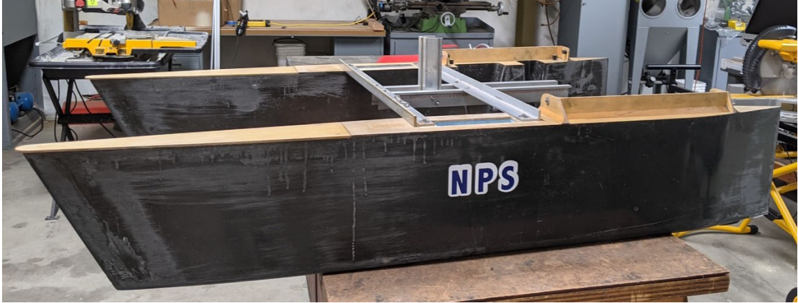
Figure 9 Current status of the construction of the drag device
