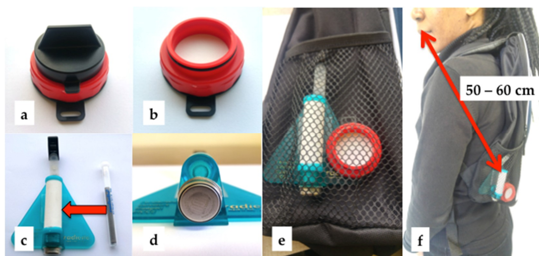
Figure A1. Photos of samplers used for personal exposure measurements: (a) Gradko rapid air NO 2 sampler (product: DIFRAM-100; UKAS method: GLM 7; detection limit: <math><0.2 \mu\text{g}/\text{m}^3</math> for 1-week exposure); (b) activated Gradko rapid air NO 2 sampler; (c) Radiello TM diffusive cartridge (right) and diffusive body attached to a triangular support plate (left) (products: Rad130, RAD120, and RAD121; detection limit for BTEX: 0.05, 0.01, 0.01, and 0.01 \mu\text{g}/\text{m}^3 , respectively; calibration: CS 2 ); (d) ACR Systems Inc. temperature logger (product: SmartButton (01-0187); detection limit: -40 \text{ }^\circ\text{C} to 85 \text{ }^\circ\text{C} ); (e) air monitoring devices in the mesh pocket of a backpack (product: Barron BB0110 Curve and Arch Design backpacks); (f) backpack worn by participants with samplers located 50 to 60 cm from the face.
