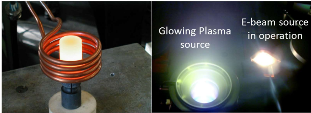
Figure 2.8: RF heated \text{LaB}_6 cathode on the left and plasma source in operation during an E-beam deposition. Photos credit to Thin Film Solutions.
