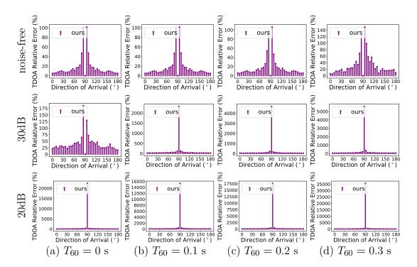
FIGURE B.1: **TDOA relative error vs DOA.** TDOA relative error (purple) for 3 different reverberation levels:  $T_{60} = \{0.1, 0.2, 0.3\}$ seconds and 3 noise conditions: noise-free, 30dB and 20dB Signalto-Noise Ratio (SNR). The results are from 10 speech signals, at 19 different locations (DOA), from 0°to 180°, with a step size of 10°. We ran 5 different simulations for each of these sources and reverberation values. The compression ratio is 40 : 1 for each signal.
