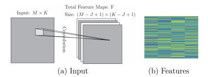
FIGURE 6.2: Convolution operation and features visualisation. CNN input matrix [4] and visualisation of this input with our data. (a) Illustrates the convolution operation when F different locals filters are used, each of size J by J. (b) Visualisation of the Input matrix M by K for one of the audio signals used for training.
