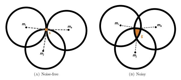
FIGURE 3.4: Spherical Least-squares (LS) error function. Represented by intersection of spheres (circles in 2D) centred at the microphones for the case in which (A) the calculations do not have noise (orange dot) and (B) when they do (orange area).
