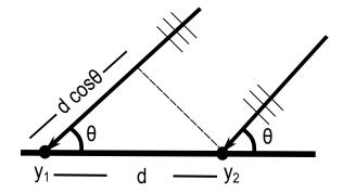
FIGURE 3.3: Planar waves reaching the microphone array from a source located on the far-field.  $\theta$  is the incident angle of the planar wave, corresponding to the DOA.
