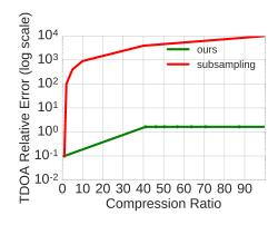
FIGURE 5.8: Subsampling vs our algorithm in a noise-free environment. TDOA Relative Error achieved for different compression ratios for a source located at Direction of Arrival (DOA) 45°. The figure shows the TDOA relative error for our algorithm (green) compared with a baseline (red) in which the signal is compressed by subsampling. We used the logarithmic scale on the Y-axis given that the error for the subsampling approach is much higher than our error.
