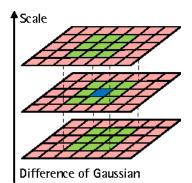
FIGURE 5.2: Local maxima/minima in DoG images. Checking the pixels on a 3 by 3 window (green) and comparing it with the neighbours above and below. The point is marked as a keypoint (blue) if it is the greatest amongst all 26 neighbours [3].
