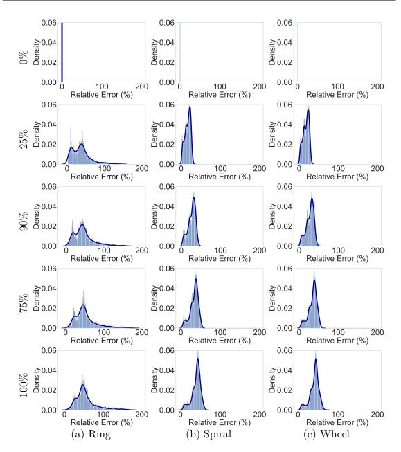
FIGURE 4.6: Relative localisation error visualised as histograms (blue) for a  $2m \times 2m$  room. Simulation of TDOA with various noise levels (0%, 25%, 50% 75% and 100%), expressed as percentages as explained in Section 4.4.1. The histograms depict the localisation error for 1600 source locations inside a  $2m \times 2m$  room. 100 estimates were averaged to determine the error estimate at each source position.
