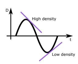
FIGURE 2.3: Relationship between the density and the gradient of the displacement. When the gradient (purple) is negative, we have a higher density value. In contrast, when the gradient is positive, we have a lower density value.
