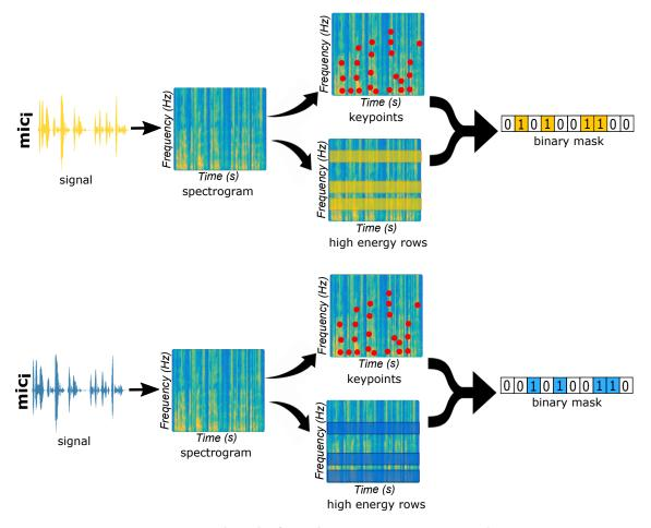
FIGURE 5.4: **Pipeline before data transmission to the Fusion Center (FC).** The signal spectrogram is computed and the SIFT keypoints are extracted. Using the steps illustrated by Algorithm 5.3.2, a binary mask is created using the extracted keypoints (yellow and blue) and the top x high energy rows. An index is filled with 1 if there is a keypoint in that position and that point lies in one of the high energy rows.
