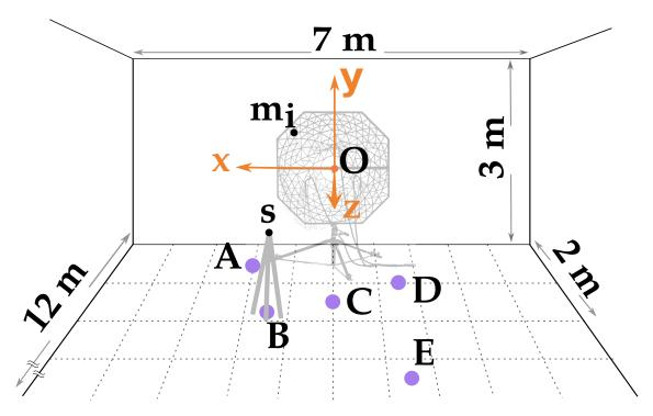
FIGURE 4.2: Experimental setup and coordinate system (orange). The room size is  $12m \times 7m \times 3m$ . The speaker was positioned, using a tripod, to be on the plane y = -0.32 for all five positions A, B, C, D and E (purple dots).
