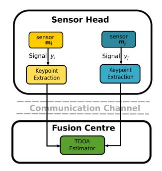
FIGURE 5.3: **Overview of the system architecture.** Keypoint extraction (yellow and blue) occurs at the Sensor-Head (SH). These keypoints are then communicated to a Fusion Centre (FC), which may be either a centralised node, or simply another sensor node, where the Time Difference of Arrival (TDOA) is calculated (green).
