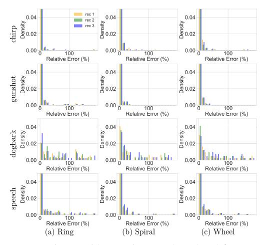
FIGURE A.1: TDOA errors for source located at A:(2.0,-0.32,0.5). Each row represents the results of a dataset: chirp, gunshot, dogbark and speech respectively. For each of them, the results for three different recordings are illustrated by the color bars. The histogram shows a larger error for the *dogbark* dataset, arising from the use of the Generalized Cross-Correlation Phase Trans-
