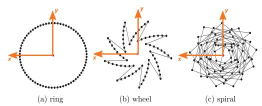
FIGURE 4.1: Microphone configurations Ring, wheel and spiral. The purple dot represents the centre of the array. The microphones are arranged in the xy plane with z = 0.
