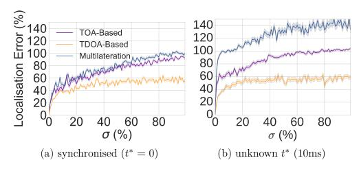
FIGURE 4.3: Relative localisation errors. Using  $O_1$  (TOA), in purple,  $O_2$  (TDOA), in orange, and multilateration [2], in blue, in the event that (a) speaker is synchronised with microphones and (b) time of emission is unknown.
