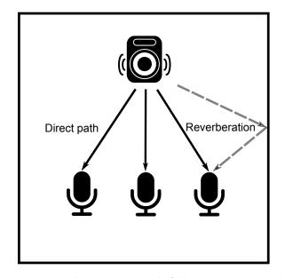
FIGURE 2.5: **Reverberation.** Path followed by a sound from the source (speaker) to the target (microphones) for a non-reverberant (black arrow) and reverberant (gray dotted arrow) situation.
