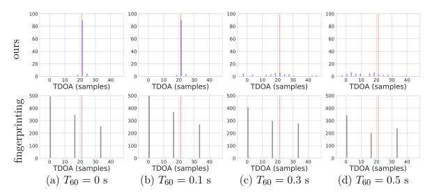
FIGURE 5.14: Our algorithm vs fingerprinting. Histogram of estimated TDOA values for a source located at (x = 2, y = 1, z = 5) and 20*dB* SNR. The ground truth of TDOA is 21.25. While our approach (blue) presents a clear peak in the TDOA distribution, the fingerprinting approach (gray) presents the highest peak at zero.
