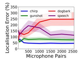
FIGURE 4.8: Localisation accuracy vs microphone pairs. Localisation accuracy for various numbers of microphone pairs. In cases of accurate TDOA estimation, such as chirp and gunshot, the curve stabilises when a relatively low number of microphone pairs (100) has been used. In the case of more challenging datasets, such as speech and dogbark, the use of fewer microphone pairs decreases the localisation error, since a large number of microphone pairs introduces more noise to the source estimation.
