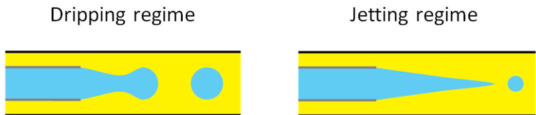
Figure 1.4 The co-flow stream design involves a capillary (grey lines) being inserted into a microfluidic channel (black lines) and the dispersed and continuous phases are injected into the two spaces respectively. Droplet formation is dependent on the flow rates of the phases; if the continuous phase flow rate is low then droplets are formed at the tip of the capillary in the dripping regime, as the flow rate is increased droplets are formed further away from the capillary in the jetting regime. Blue represents the dispersed water phase while yellow represents the continuous oil phase.
