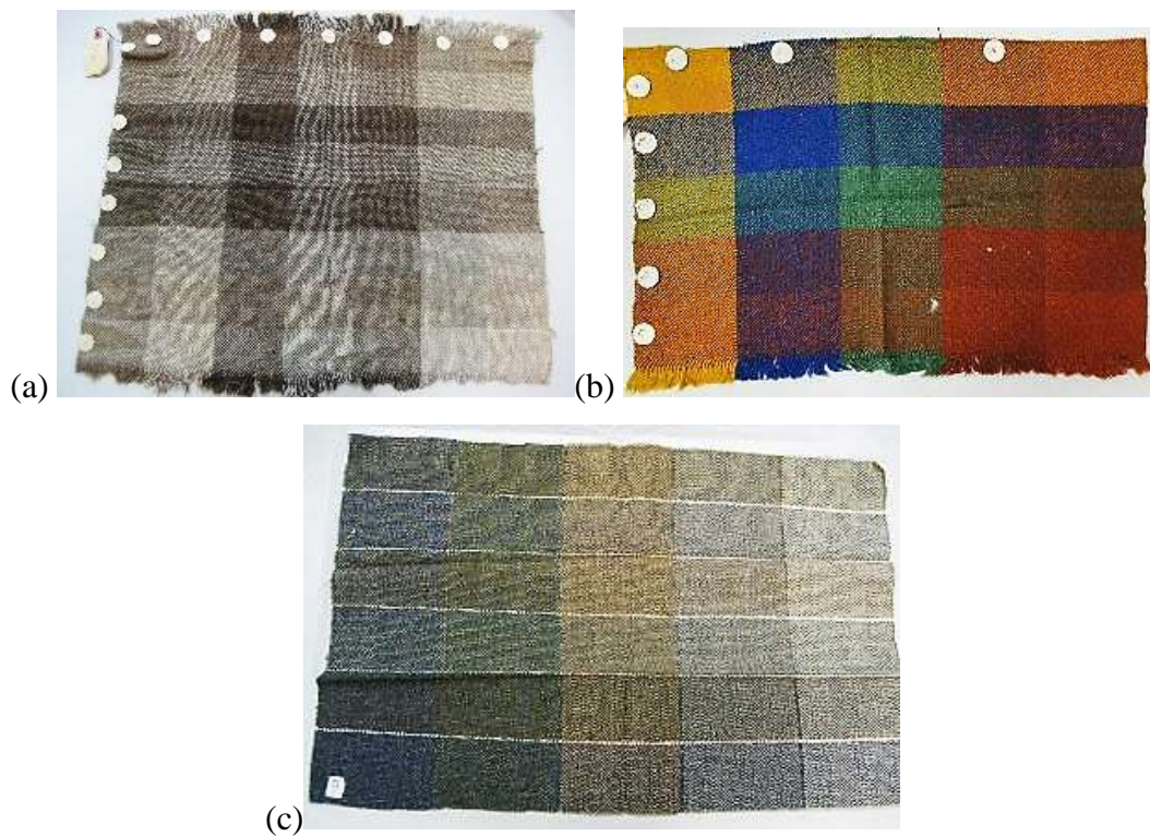
Figure 3.17 examples of blending within a warp and weft in TMA range cloths: (a) using natural shades, (b) using dyed colours, (c) using mixtures 1930s-1960s (2011)
