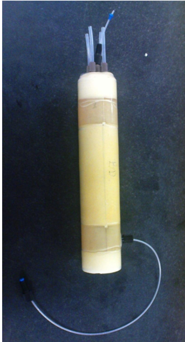
Figure 70: Flow cell with BD sample. The bottom tube connects to the inlet slit, whereas the top tubes comprise the fluid outlet for the fracture and the drainage outlets for the rock matrix.
