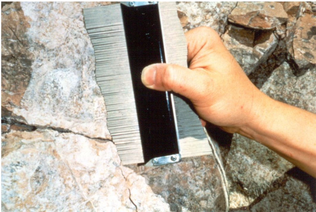
Figure 5: A Barton Comb, here being used in a field measurement, is a profile gauge commonly used for the classification of roughness profiles of rock surfaces. Joint roughness coefficients (JRC) for the surface can be determined by comparing the fracture surface geometry with Barton's standard profiles — cf. Barton and Choubey, 1977 [14]. (Image from Hubbard Brook Ecosystem Study [87]).
