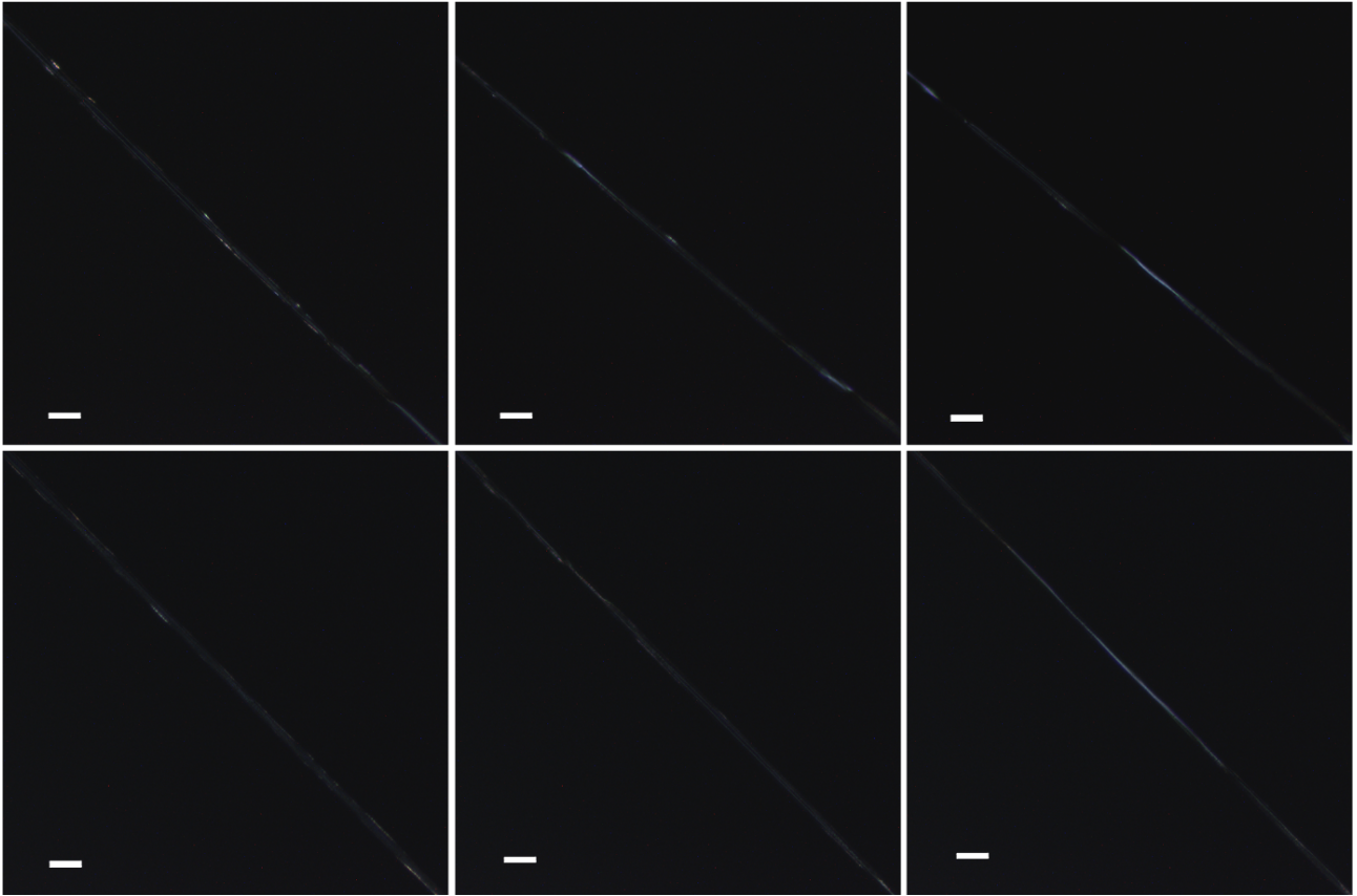
Supplementary figure 11. Polarized microscopy images of NT2RepCT fibers. Images were captured before (upper row), and after (lower row) 2h incubation at 85% humidity. Scale bars equals 50 micrometers.
