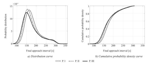
Figure 7 – The fitting curves of the final approach interval
