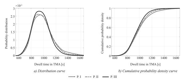
Figure 6 – The fitting curves of dwell time in TMA
