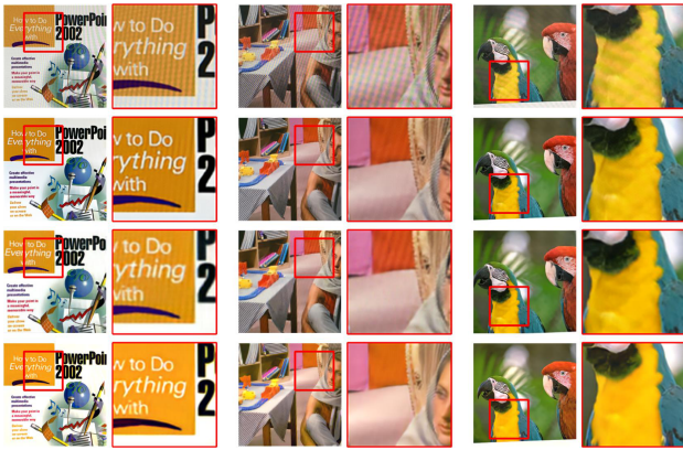
Fig. 12. Visualized results produced by MBCNN on real moiré images. From top to bottom are the input moiré images, and the results of MopNet, WDnet, and MBCNN. The moiré images are captured with iPhone6S and AOC 27B2H.
