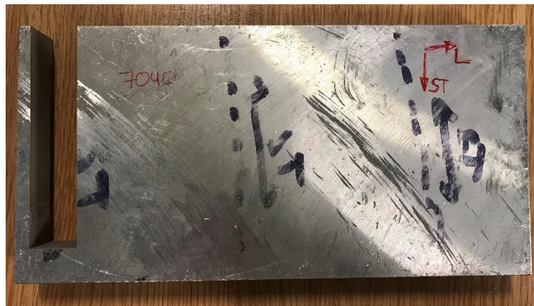
Figure 4-1. Blocks of the as-received wrought commercial alloy AA7040-T7651
