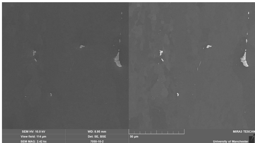
Figure 6-7. BSE-SEM image of sample 3 after polishing, and before tensile testing at high humidity. After this step, the surface is smooth, with no apparent corrosion products on the surface.
