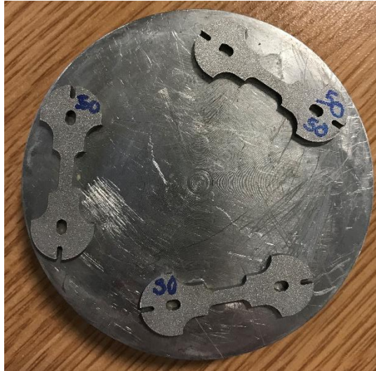
Figure 4.4. Samples stuck to a polishing wheel; this method ensures that all samples mounted will have a similar thickness for posterior analysis.
