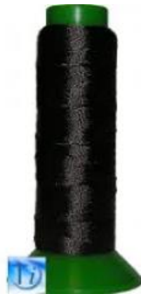
Figure 2-2. Non-metallic coated sewing yarns (TIBTECH, Carbon Tenax) [32]
