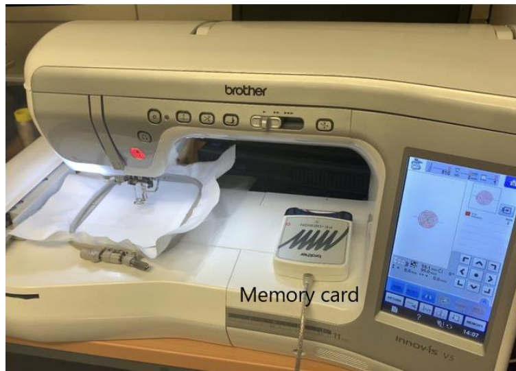
Figure 3-2. Embroidery machine (Brother IS-V5) and the memory card
