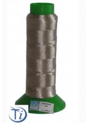
Figure 2-1. Metallic coated sewing yarns (TIBTECH, Silverpam 250) [32]
