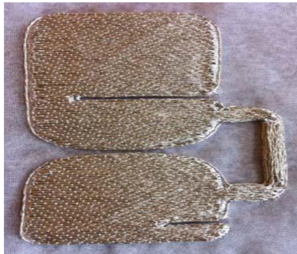
Figure 2-26. Double stitching structure [33]
