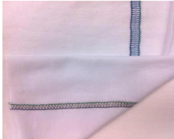
Figure 2-31. Embroidered strain sensor [101]
