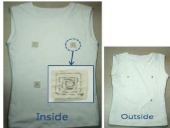
Figure 2-34. ECG shirt with embroidered ECG electrodes [103]
