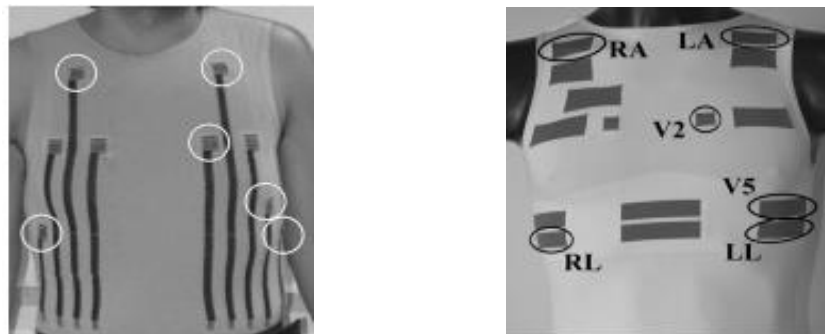
Figure 2-15. (Left) Flat knitted fabric electrodes, (Right) Seamless knitted fabric electrodes [77]
