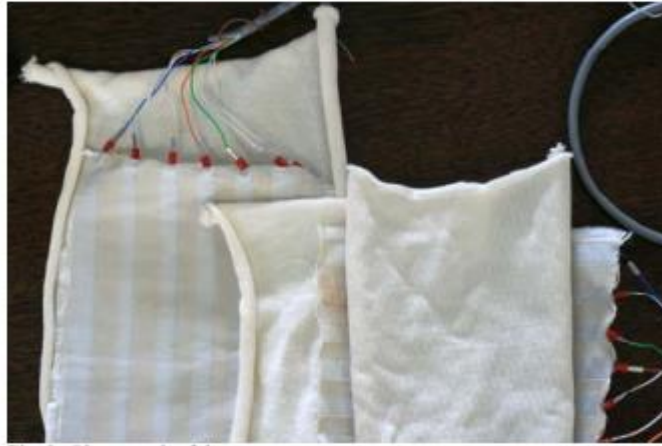
Figure 2-61. Textile moisture sensor matrix [173]
