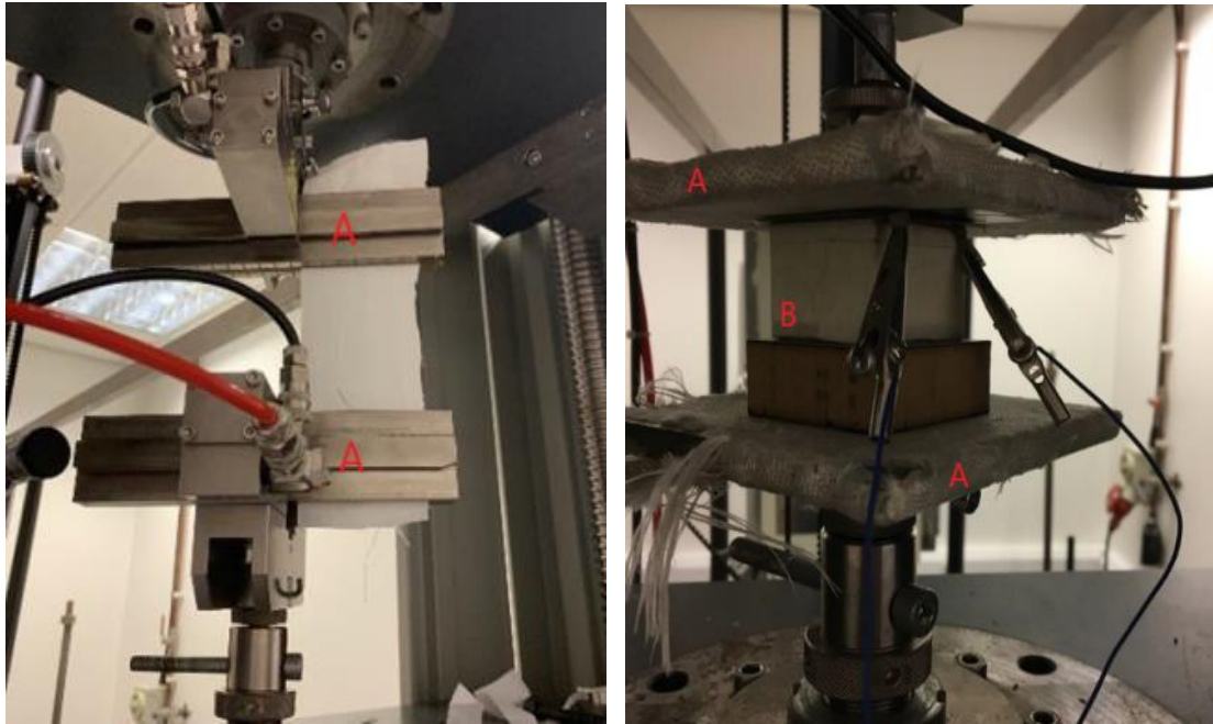
Figure 3-6. (Left) Machine during tensile test, A is the gripper. (Right) Machine during compression test, A is the compression board and B is the wooden cube
