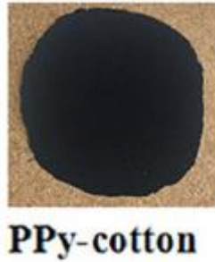
Figure 2-74. PPy-Cotton heating element [190]
