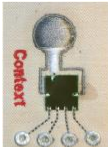
Figure 2-21. Embroidered contactless sensor [27]
