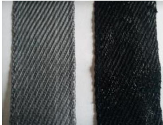
Figure 2-49. Woven fabric before and after being coated [161]
