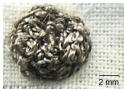
Figure 2-16. Textile electrode obtained by moss embroidery [79]
