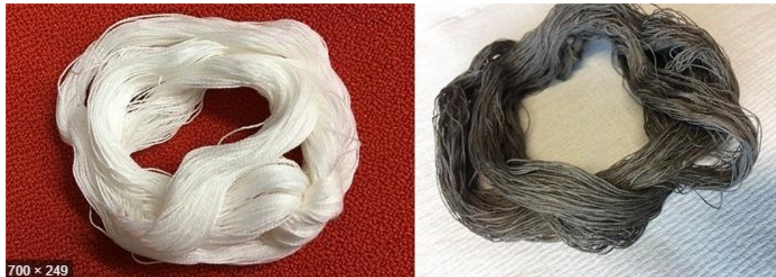
Figure 1-2. (left) Uncoated yarn, (right) graphene coated yarn [10]
