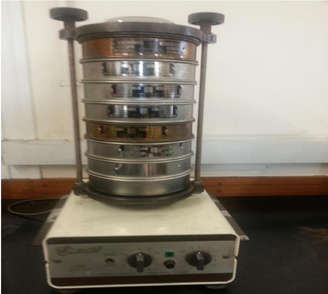
Figure 4.3: A 7 Tray-Laboratory Test Sieve Shaker
