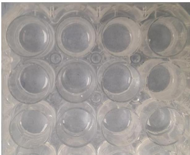
Fig: 4.13: Mould used to prepare PDMS encapsulated samples
