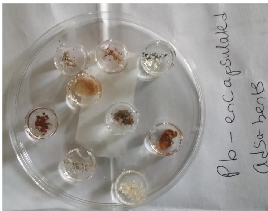
Figure 10.4: Photographs of Pb(II) PDMS encapsulated samples
