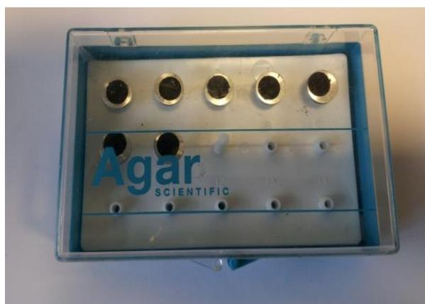
Figure 4.11: SEM samples for analysis mounted on SEM pin stubs.
