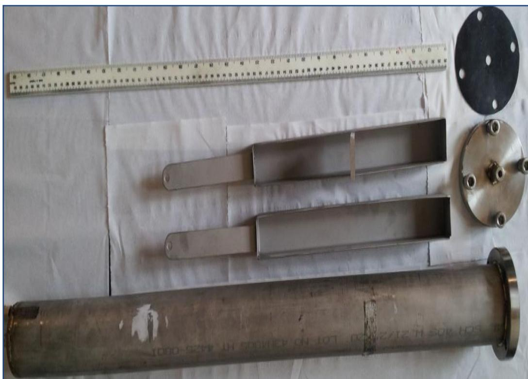
Figure 4.5: Stainless Steel Sample Holder and Horizontal Steel Tubular Reactor used for pyrolysis.
