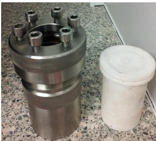
Figure 4.9: Teflon lined autoclave
