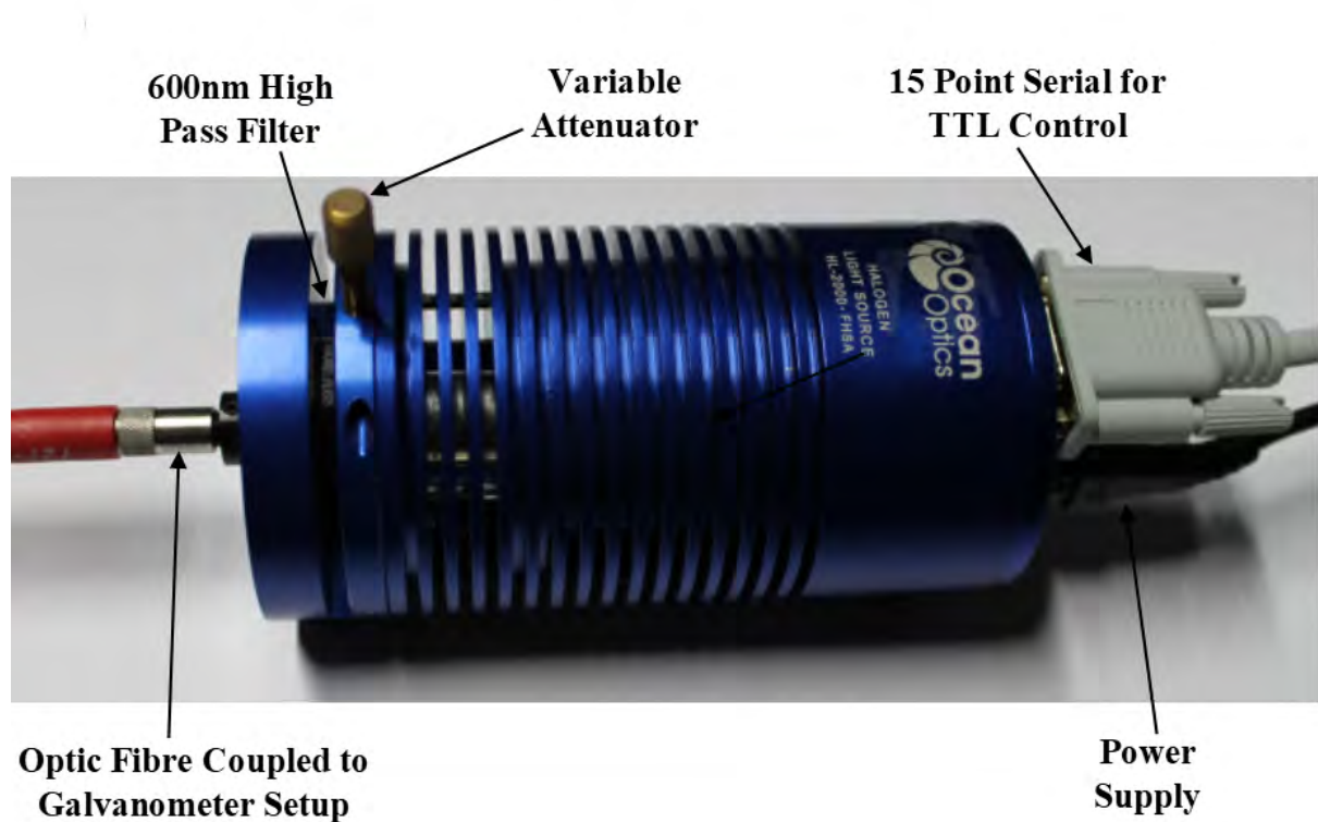
Figure 3.4: Photograph of the light source with the 600nm high pass filter added.
