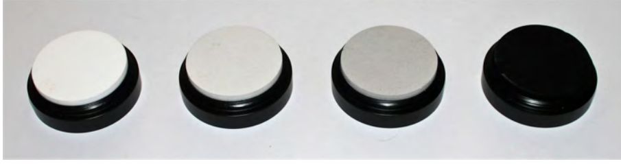
Figure A.4: Diffuse reflectance standards with either 99%, 50%, 25% or 2% from left to right.
