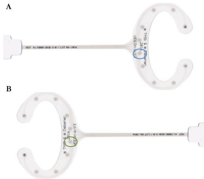
Figure 3.2 cEEGrids (A) Right cEEGrid with ground electrode R5 circled in blue. (B) Left electrode with reference electrode L6 circled in green. Image retrieved from: http://ceegrid.com/home/concept/ . The image has been modified for illustrative purposes.
