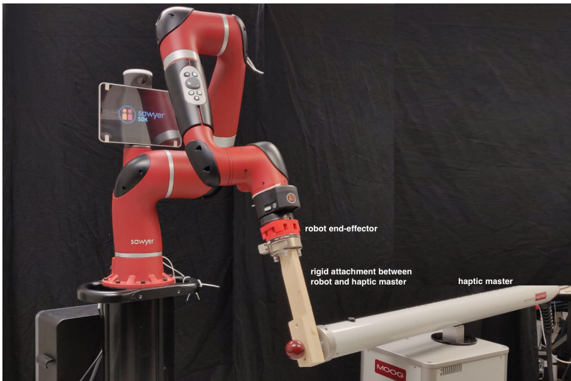
Figure 5.11: Porridge experiment setup. The porridge environment is emulated on the Moog Haptic Master. Sawyer's end-effector is initially aligned with the tip of the haptic device and connected using a wooden plank. The maximum drag force generated by the haptic device is within the limits ( 50N) of Sawyer.
