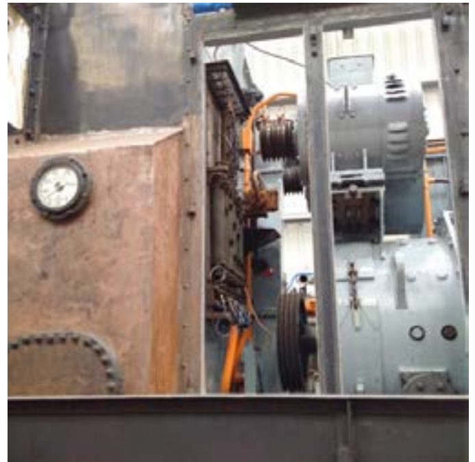
Figure 3: Detail view of a partially disassembled Class 08, showing old fashioned electrical equipment (author's collection).
