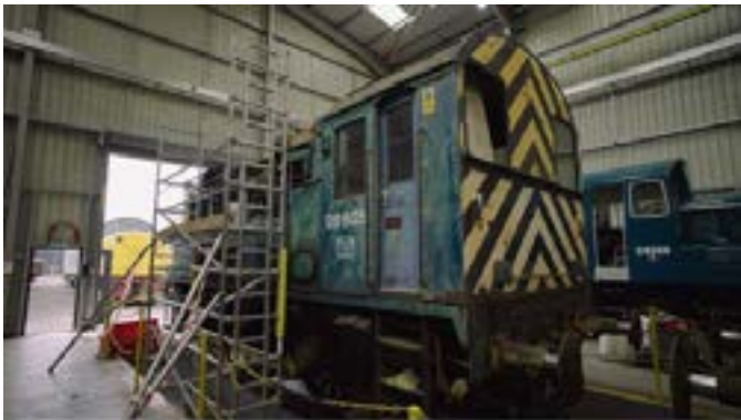
Figure 6: HydrosHunter: Diesel locomotive set to be converted to hydrogen power (Severn Valley Railway).
