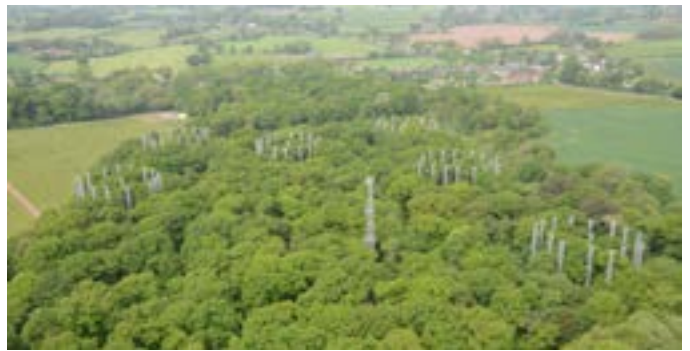
Figure 1. The Free-Air CO 2 Enrichment facility of the Birmingham Institute of Forest Research: BIFoR FACE, one of the three largest climate-change experiments in the world. Three of the patches surrounded by the metal infrastructure receive elevated CO 2 (150 ppm above an ambient level which is currently ~410 ppm). The other three, 'control', patches receive unaltered ambient air. Photo courtesy of Prof. Jo Bradwell.
