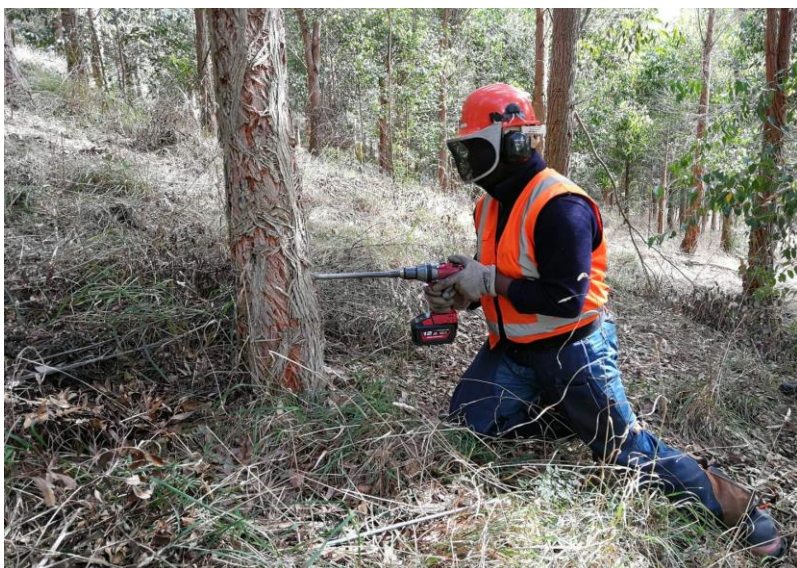
Figure 3. Coring an E. globoidea tree using a light weight battery powered corer.
