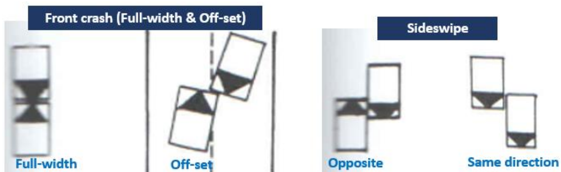
Figure 3: Crash configuration (first impact), Bukit Aman Traffic Investigation and Enforcement (JSPT) Royal Malaysia Police
