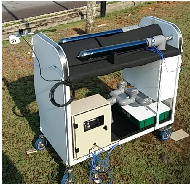
Fig. 4. The outdoor experiment between EGATC air heater and HP ETC air heater
