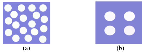
Figure 2. Varying permittivity technique: (a) increasing number of holes, (b) enlarging size of holes
