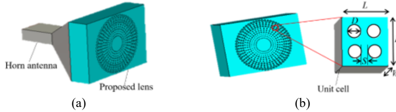
Figure 4. (a) Full model of proposed flat lens attached with pyramidal horn antenna, (b) Lens design based on unit cell
