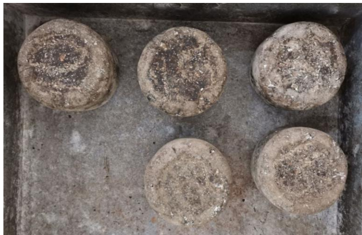
Figure 3. The sample after 300 revolutions in LA abrasion
