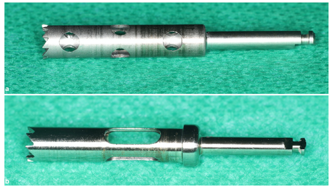
Fig. 2. The trephines used in the study. (a) the conventional trephine used in the control group; (b) the endo-trephine used in the study group. Note that the body of the instrument widens at the proximal end to form a shoulder. When this shoulder (the stop) meets the outer rim of the guiding tunnel of the surgical template, it prevents the instrument from being introduced any deeper (see also Fig. 3b).
