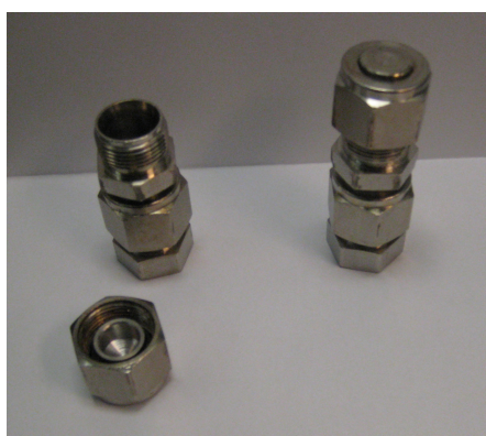
Figure 10. Reactors used for catalyst screening ( V_{\text{reactor}} = 2 \text{ mL} ).
