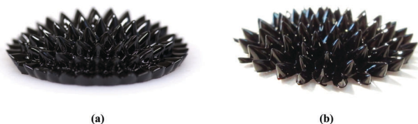
Fig. 1 Normal field instability “spikes” of the water based magnetic fluid samples on a permanent magnet (NdFeB): (a) with electrostatic stabilization; and (b) similar with electro-steric stabilization.
